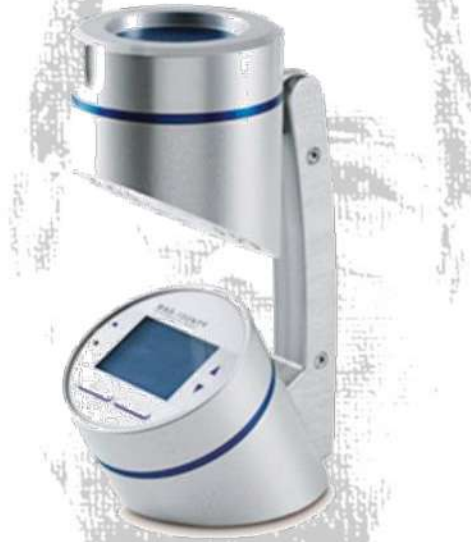
Gambar 27: microbiology air sampler merk MERCK tipe MAS 100 NT Sumber: dokumen pribadi
